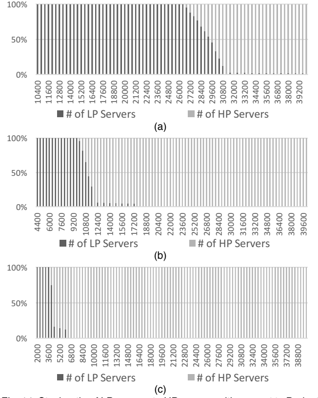
Fig. 14. Stack ratio of LP servers to HP servers with respect to Budget in (a) high, (b) medium, and (c) low traffic.
